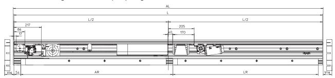
Illustrated: left hand slide to open, passage width 1065 mm
